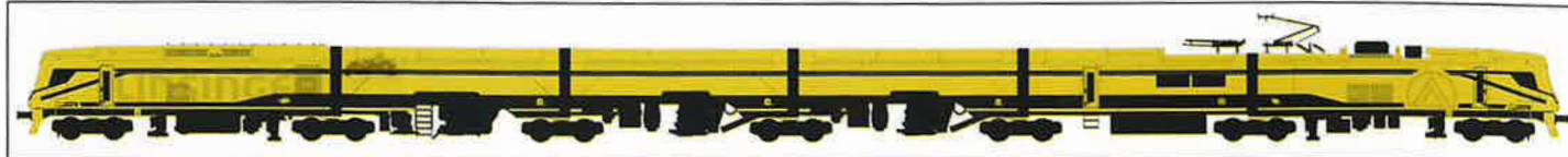
Above: Diagram of the Linsinger Railmaster rail milling machine.
