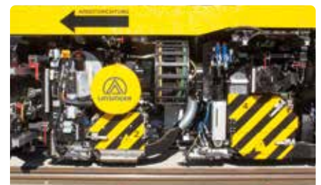
Milling unit with downstream peripheral grinding unit for maximum surface
