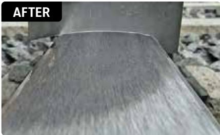
Perfect rail head reprofiling with LINSINGER rail milling technology.
