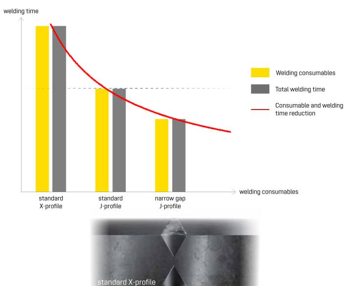
Edge milling technology allows cost savings.
