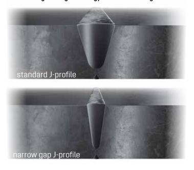
The reduction of welding joint volume minimizes the costs of consumables and increases production speed.
