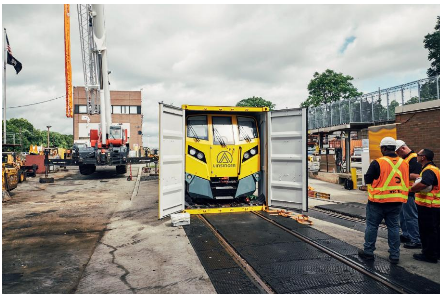
Fig. 2: Milling machine MG11 in a 40-foot container just before the railing in the depot of NYCTA
