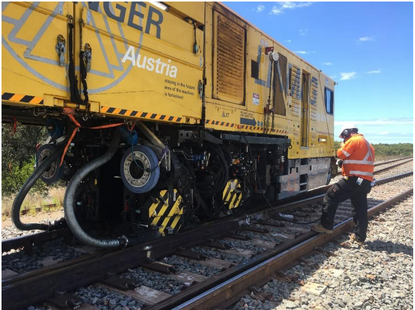
Fig. 5: The LINMAG two-way vehicle "SF02W-FS Truck" processing a switch in the ARTC network in Australia.
