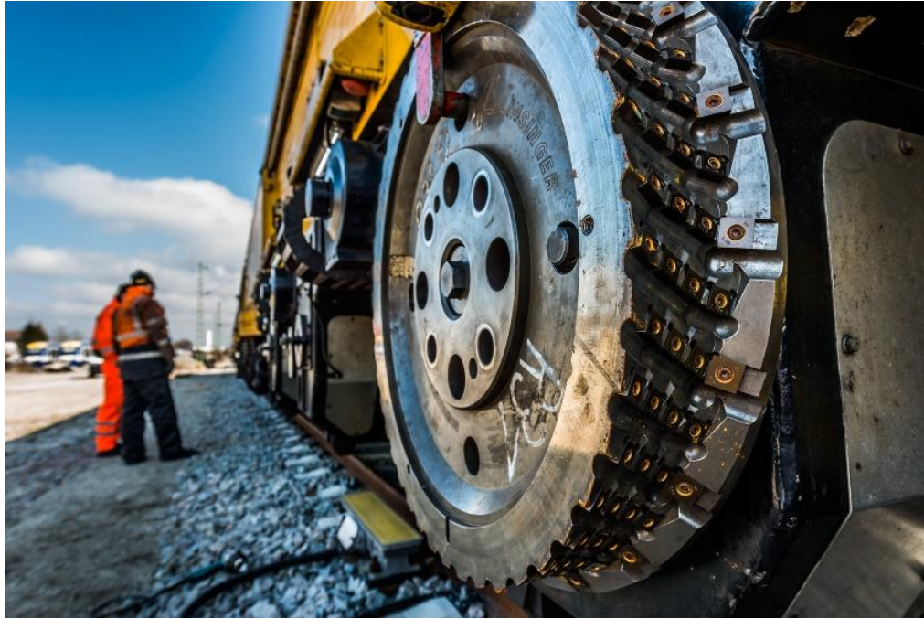
Fig. 1: LINSINGER milling wheel on a high performance mill MG31. The milling wheel design is optimised for maximum productivity and tool life.
