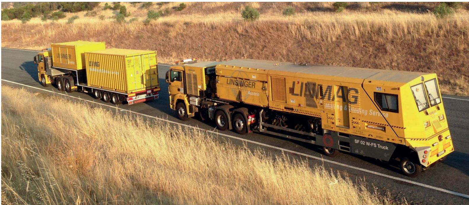
Fig. 3: Rail-Road-Truck SF02W-FS (operated by Linmag Australia Pty. Ltd) with included workshop and spare parts container
