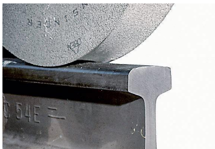
Fig. 1b: Circumference grinders for adjusting a noise optimised surface finish
