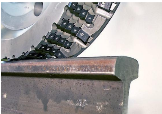
Fig. 1a: Circumference milling wheel for re-profiling the rails and completely remove damages
