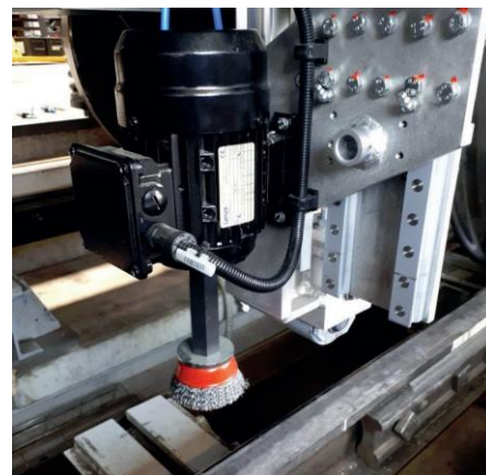
Fig. 1c: Rotating wire brush for later cleaning of the rail surface
