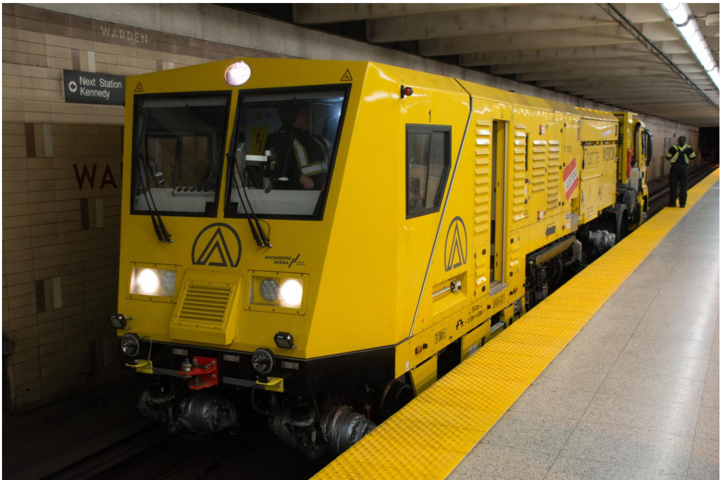
Fig. 3 Milling-Truck SF02W-FS at Warden Station at the TTC subway.
