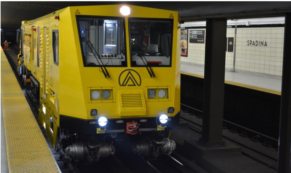
Fig. 3: Rail milling truck SF02W-FS (operated by Rhomberg Sersa Canada Ltd.) during rail processing at Toronto's underground.
