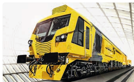
MG31 High-speed rail processing on mainline railways
